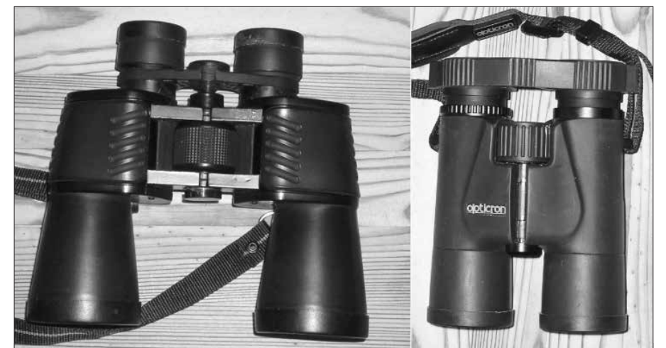
Samples depicting Porro Prism binoculars on the left and Roof Prism binoculars on the right.
