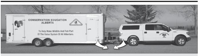
Without weight distribution. Note how the weight of the trailer is carried forward toward the front of the trailer and the rear of the truck.
