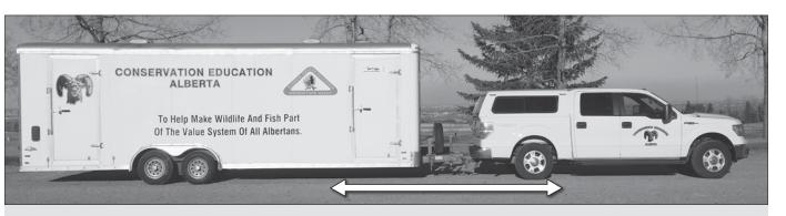
With weight distribution bars. Note how the weight of the trailer is more evenly distributed.
