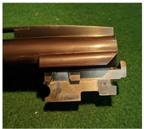
The information on this barrel shows 34\*. The 34 indicates the barrel length and the single \* for this manufacturer indicates Full Choke.
